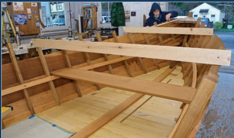
Student Kendra (K) Woolfe works on fitting the white oak breast hook on the Port Hadlock Work Skiff.
