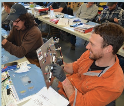
Students Adam Snider (foreground) and Shawn Meyer practice applying Click Bond wire supports on a wire management board.
