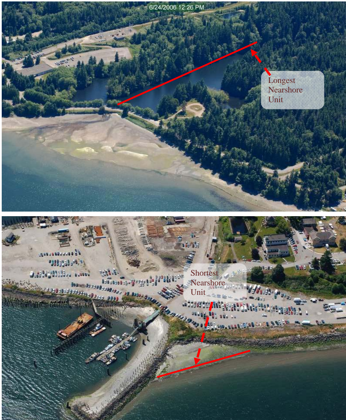
Figure I-3. Ecology Shoreline Obliques 2006. These capture both the longest NAU (top) and the shortest (bottom). Note that the longest shoreline unit is measured by the length of shoreline around the inlet, not the vertical length.
