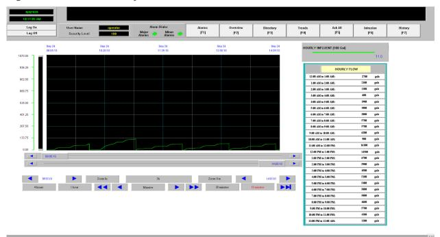
Figure 4-11. KWWTP hourly influent trend HMI screen
