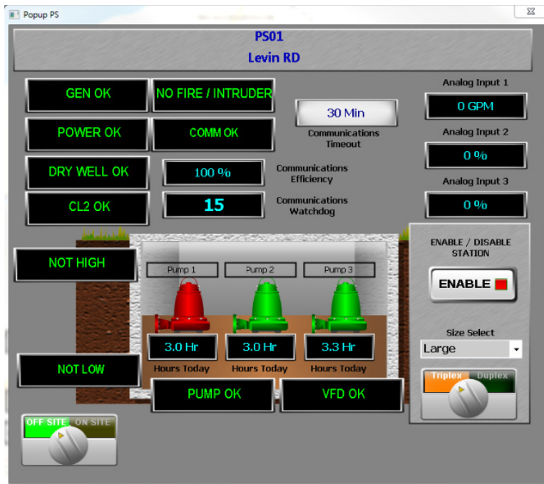
Figure 4-9. Example pump station pop-up HMI screen
