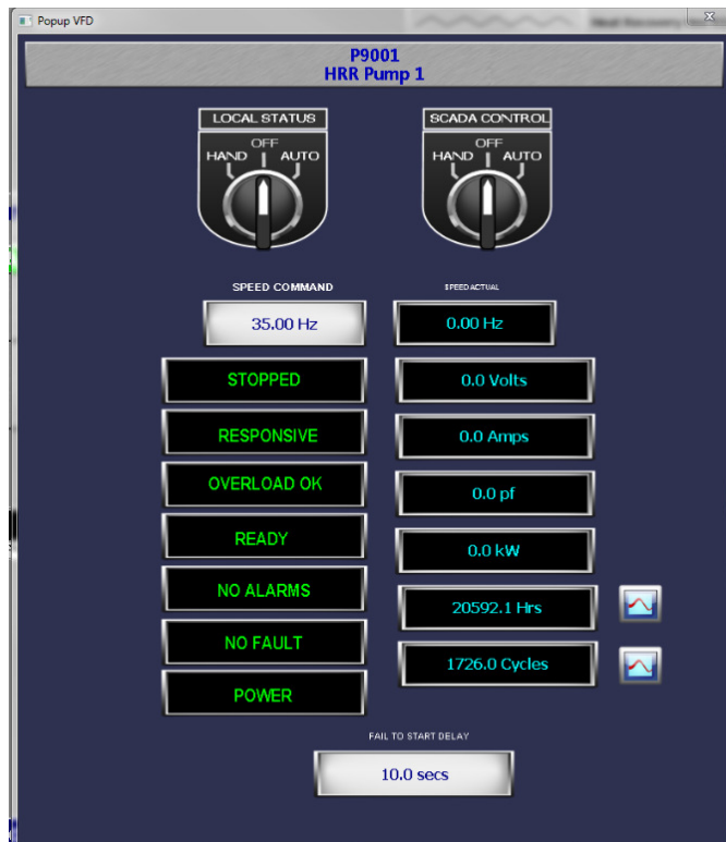
Figure 4-10. CKTP HRR pump 1 equipment pop-up window
