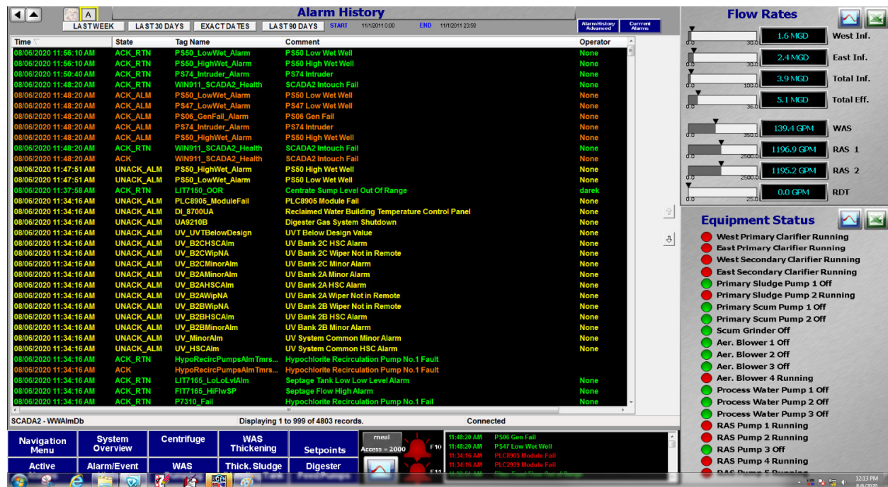
Figure 4-12. CKTP alarm history HMI screen
