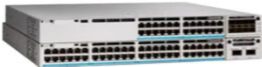
Figure 3-2. Cisco Catalyst 9000 family switch
