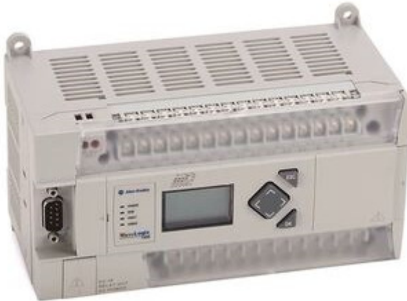
Figure 3-2. Allen-Bradley 1766-L32BXBA MicroLogix 1400 PLC
