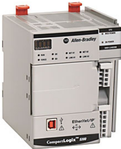
Figure 4-2. Allen-Bradley 5069-L320ER CompactLogix 5380 controller
