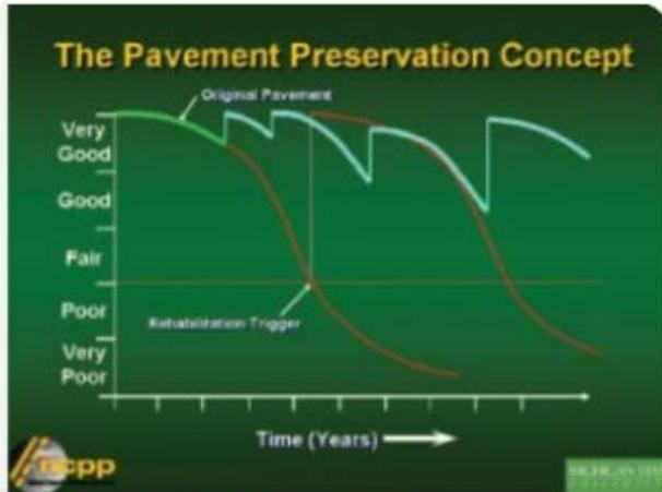
By applying pavement maintenance at frequent intervals existing pavement (green) condition can be prolonged over many years (blue), as opposed to letting the pavement decline over years to a point where major expenditures are required (red).
