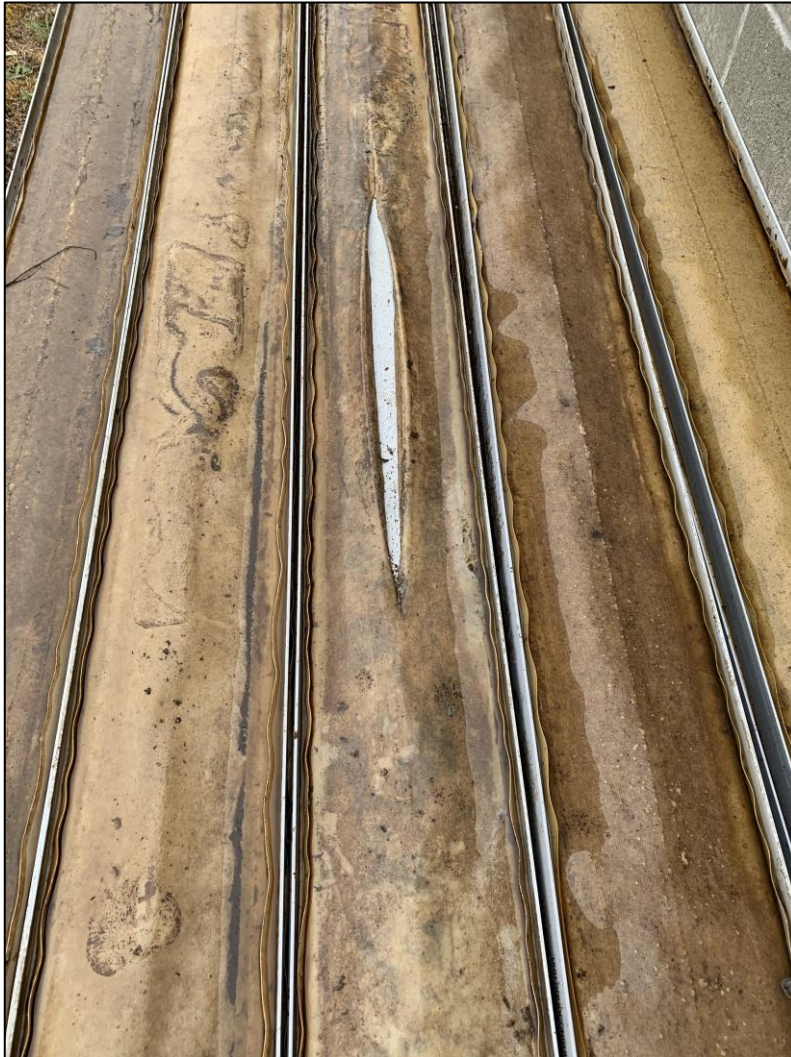
Figure 1 Failed Strip Diffusers at Central Kitsap WWTP
