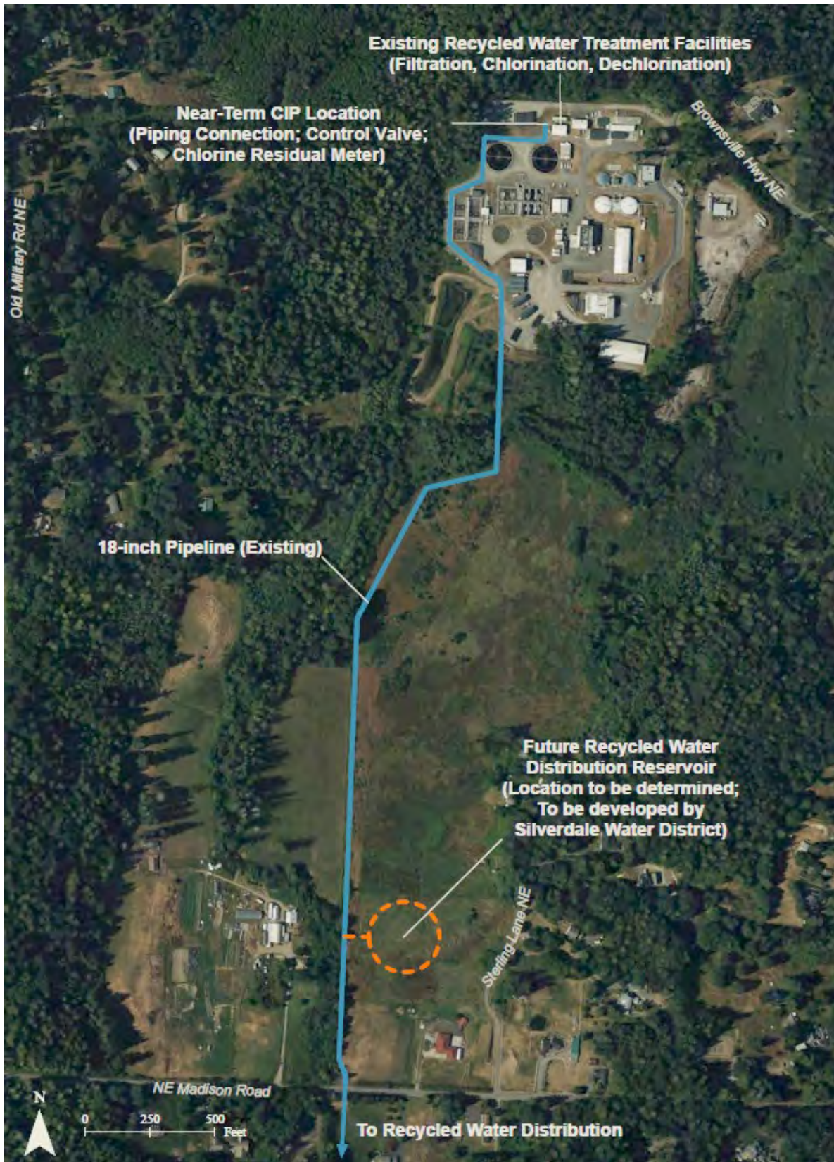
Figure 9-2 | Near-Term Recycled Water Treatment/Distribution Components
