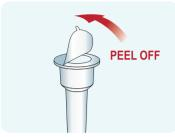
Peel off aluminum foil seal from the top of the extraction vial containing the extraction buffer.
