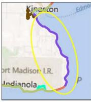
Net shore drift showing left-toright sediment transport (in this case, from south to north) in drift cell
