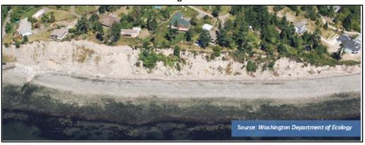
Typical Shoreline Slope and Development in Deep-Seated Landslide Reach
