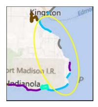
Sediment source mapping delineated three shallow landslide reach (blue) and a deep-seated landslide reach (gray), as well as one mixed landslide reach
