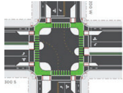
Figure 4.3 The 2018 S-TIS recommends a strategy of protected intersections and separated bike lanes to provide low-stress facilities for bicyclists
