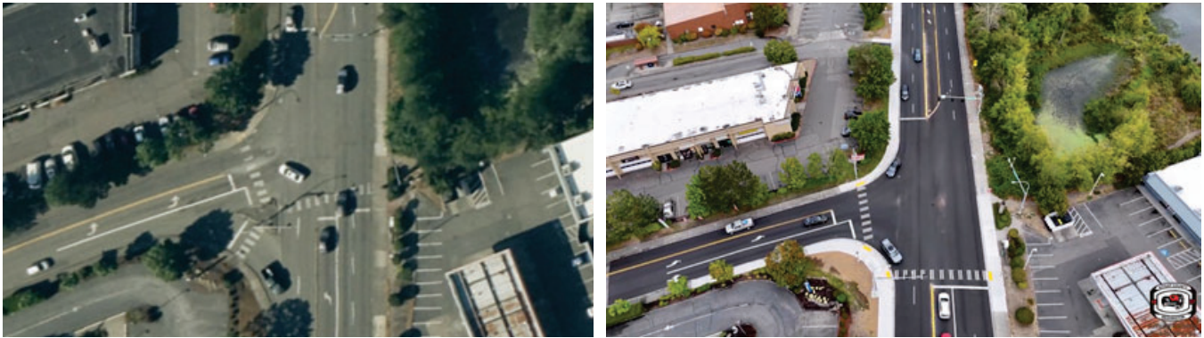
Figure 4.5 Before and after images showing removal of slip lane, new sidewalks, and curb ramps at the intersection of Silverdale Way and Randall Way
