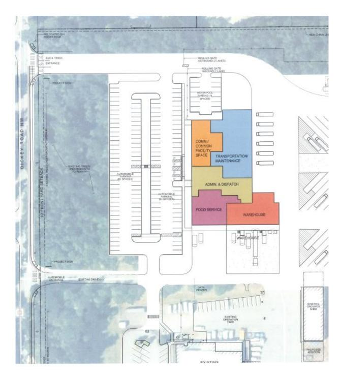
Central Kitsap Transportation and Warehouse Floor Plan and General Site Plan
