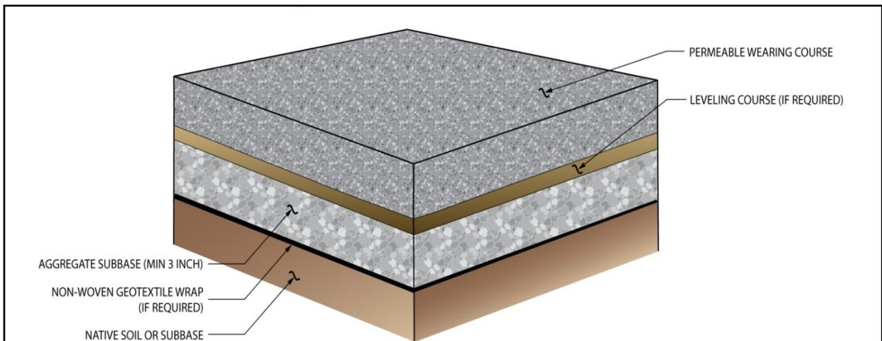
*Figure 2.1: Typical Permeable Pavement Surface Section*
