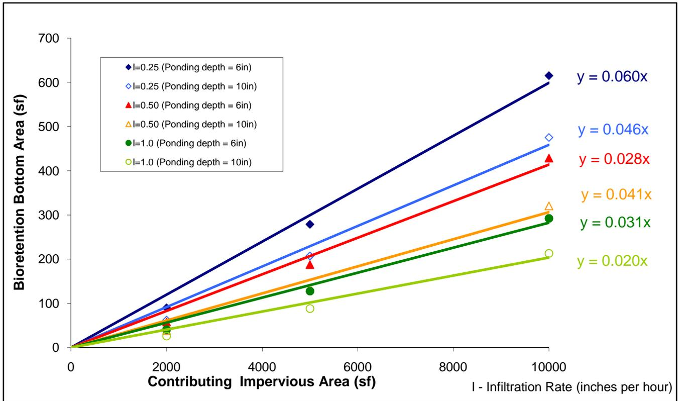
Figure C6. Bioretention facility (bottom area) sized for water quality treatment as a function of contributing impervious area (annual precipitation of 36 inches).
