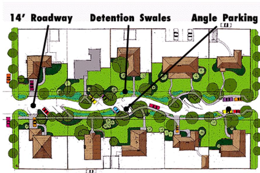
Figure 14.1: Schematic of a section of the SEASTreets Layout. Source: Seattle Public Utilities
