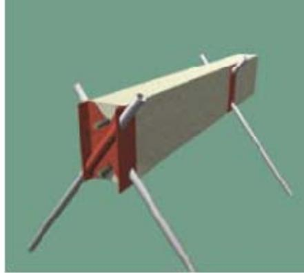
*Figure 20.1: A typical minimal excavation foundation wall section.*
