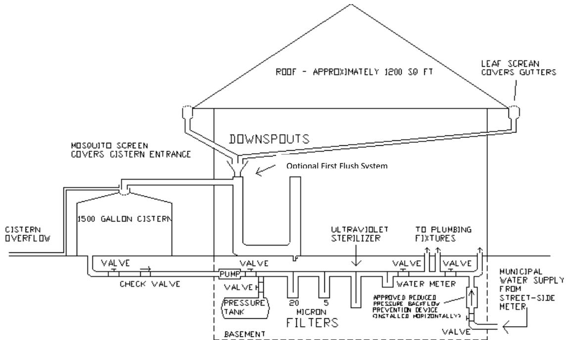
Figure 8.1: Typical Roofwater harvesting system. Source: Experiments in Sustainable Living
