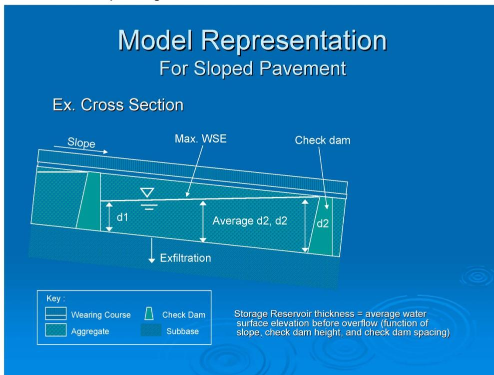
Figure 4.3: Modeling representation of sloped base storage with check dams
