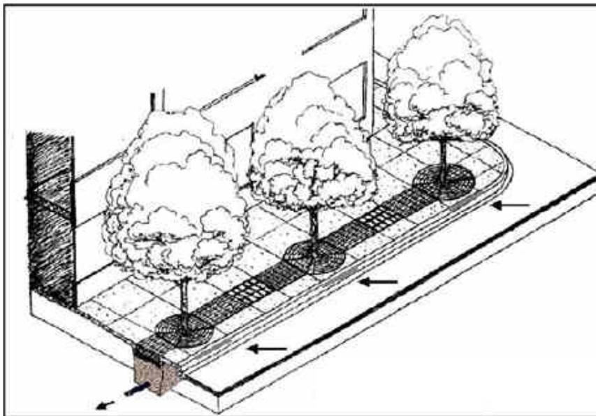
Figure 18.4: Manufactured Tree Box Filters For Stormwater Management
