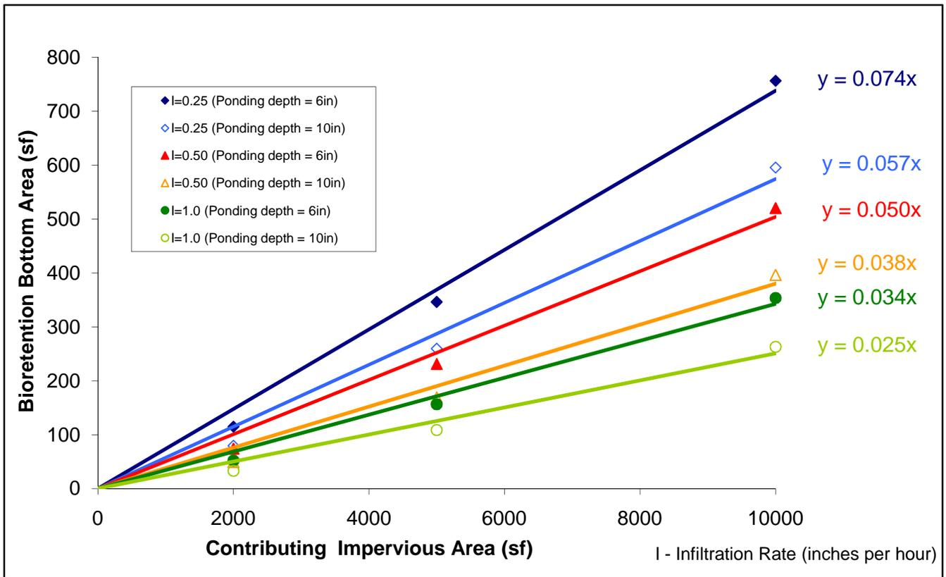
Figure C7. Bioretention facility (bottom area) sized for water quality treatment as a function of contributing impervious area (annual precipitation of 44 inches).
