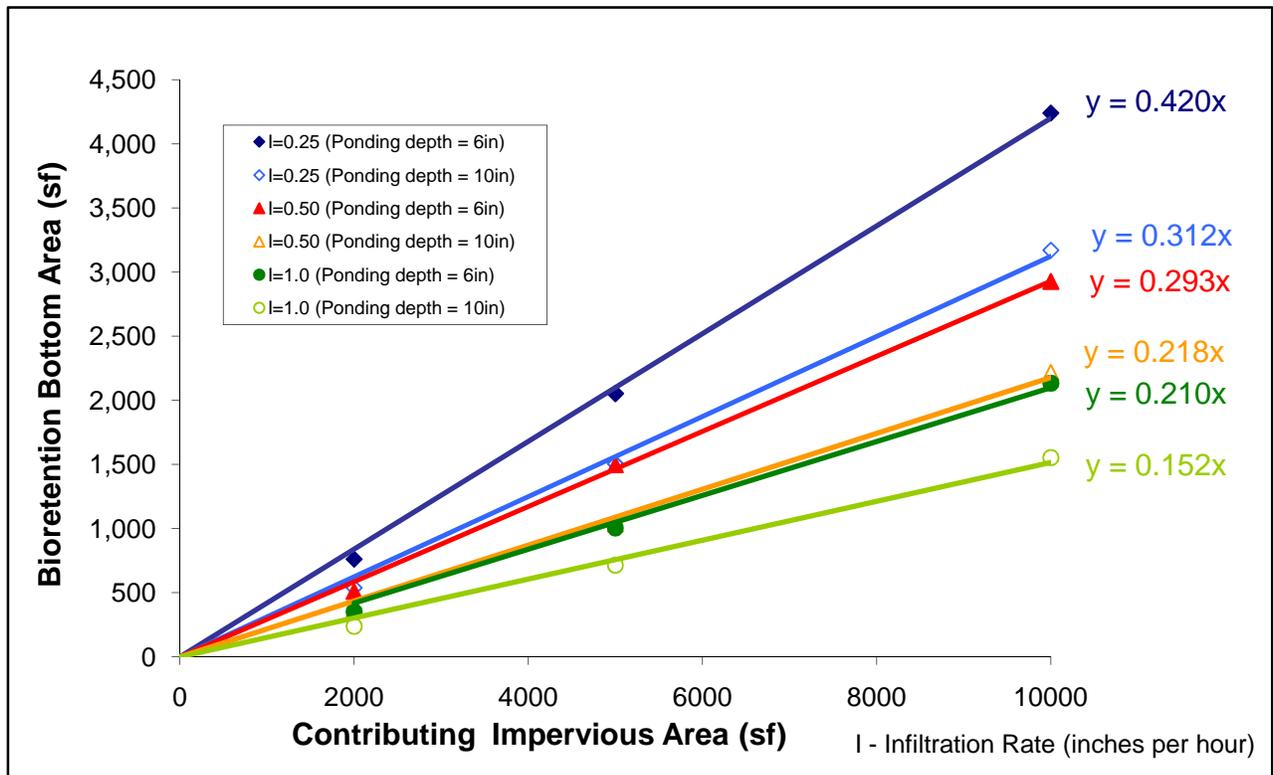
Figure C4. Bioretention facility (bottom area) sized for flow control as a function of contributing impervious area (annual precipitation of 52 inches).
