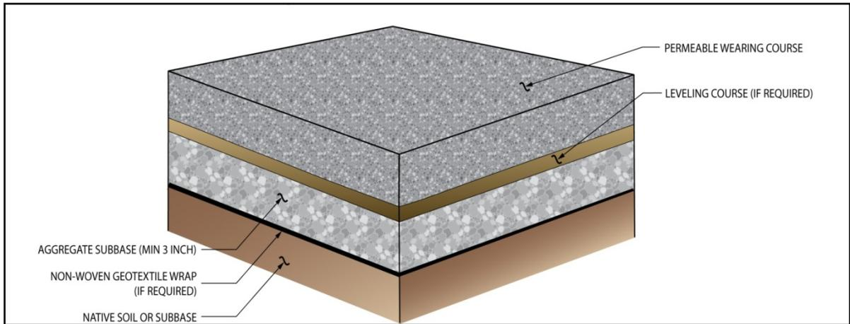
Figure 1.2: Typical Permeable Pavement Surface Section
