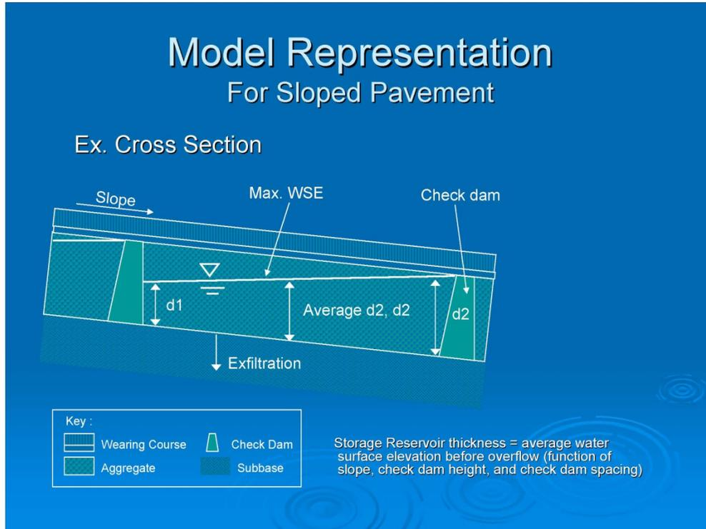
Figure 3.4: Modeling representation of sloped base storage with check dams
