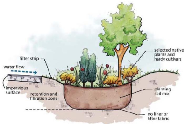
Figure 9.1: Bioretention cell or raingarden – allowing for 100% infiltration or evaporation of inflowing stormwater
