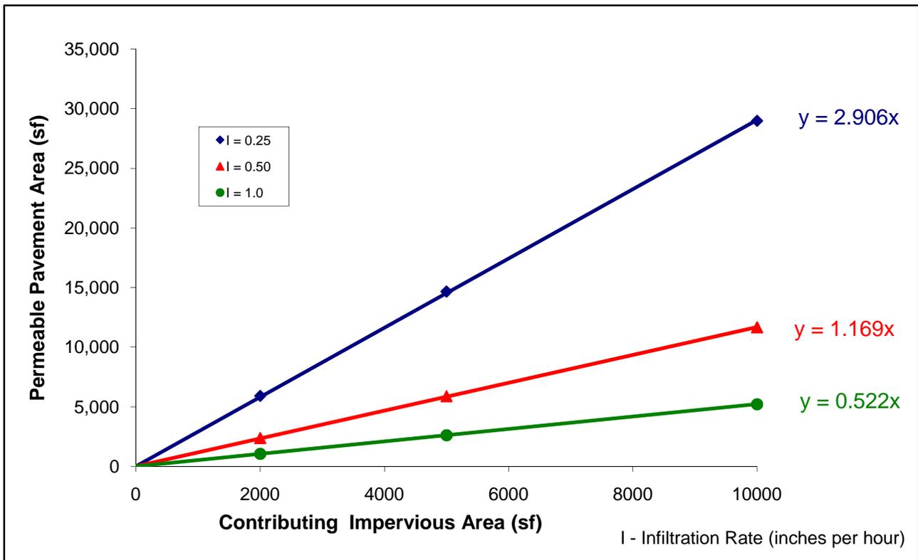
Figure C10. Permeable pavement facility sized for flow control as a function of contributing impervious area (annual precipitation of 36 inches).
