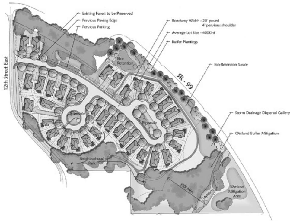
Figure 17.1: Meadow on the Hylebos site plan (LID Technical Guidance Manual2005)
