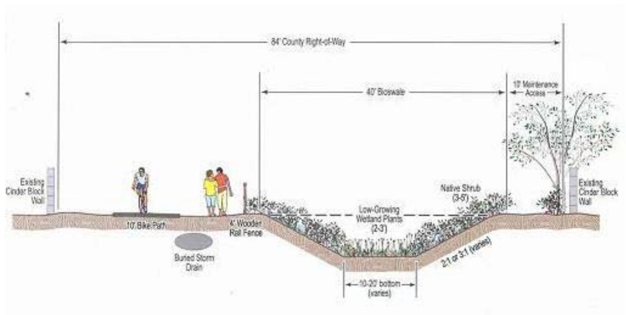
Figure 9.3: Cross section of a linear bioretention cell or swale – allowing for 100% infiltration or evaporation of inflowing stormwater
