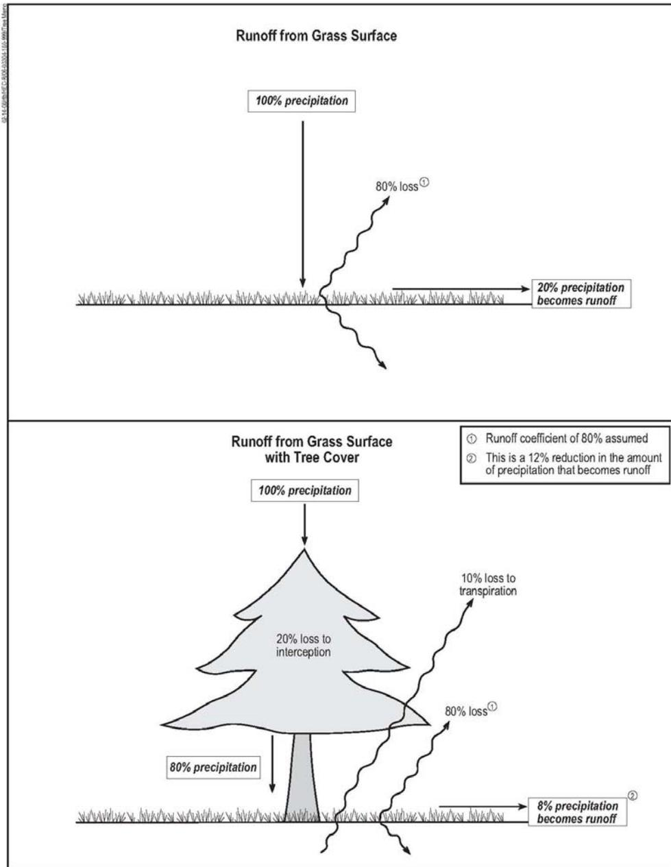
Figure 10.2: Conifer with underlying grass on till surface versus grass on till surface with no
