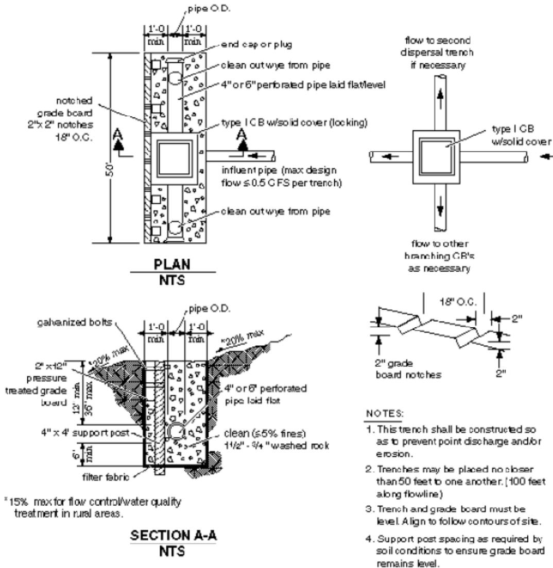
Figure 5.2: Details of a standard dispersion trench with a notched grade board for dispersing concentrated stormflows across a slope.
