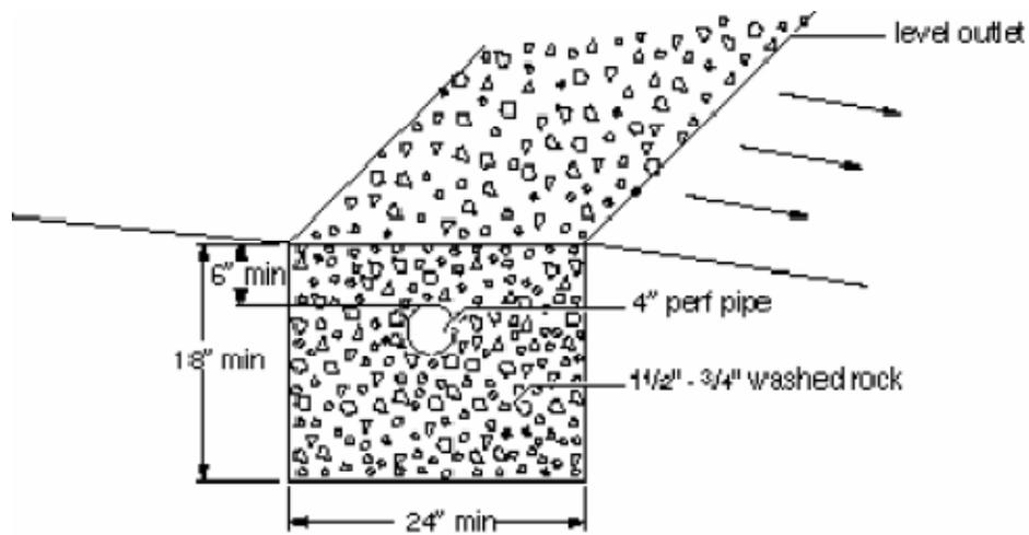
Figure 5.1: Cross section of typical level spreader trench for infiltrating and/or dispersing stormflows across a slope. Note the level outlet at the down-gradient lip of the trench to prevent concentrated flows. (From SMMWW Vol 5)
