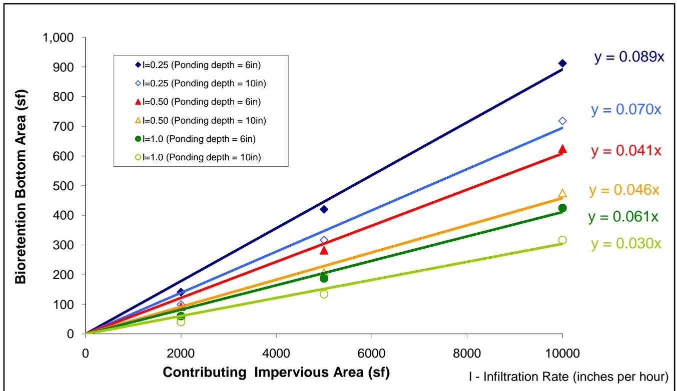
Figure C8. Bioretention facility (bottom area) sized for water quality treatment as a function of contributing impervious area (annual precipitation of 52 inches).
