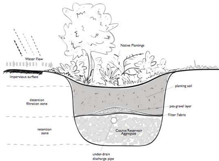
Figure 9.2: Bioretention cell or raingarden with underdrain – typically used where slower infiltration rates or space constraints prevent the sizing of facilities to manage peak design flows. Drain is elevated above bottom of cell to allow full infiltration of typical events, with overflow relief for larger events.
