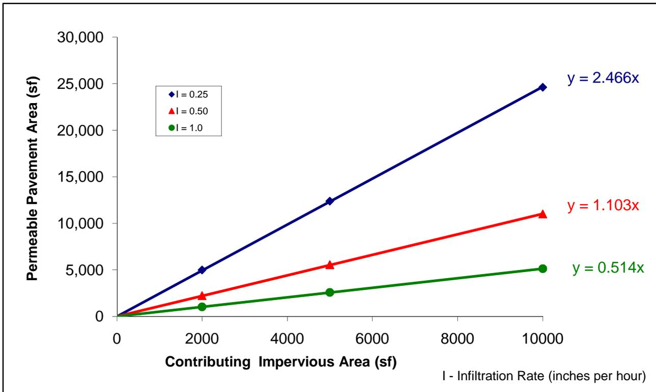
Figure C9. Permeable pavement facility sized for flow control as a function of contributing impervious area (annual precipitation of 32 inches).
