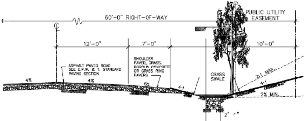
Figure 15.3: A rural residential right-of-way section has the same 60-foot width, but reduces paving width by 33% to 24 feet, and eliminates the use of concrete curb and gutter
