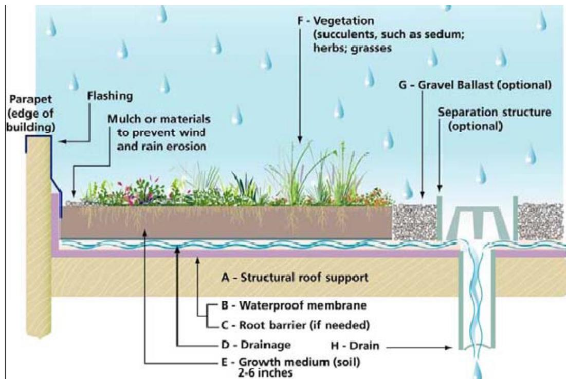
Figure 7.1: General system assembly of vegetated roof. Source: NA
