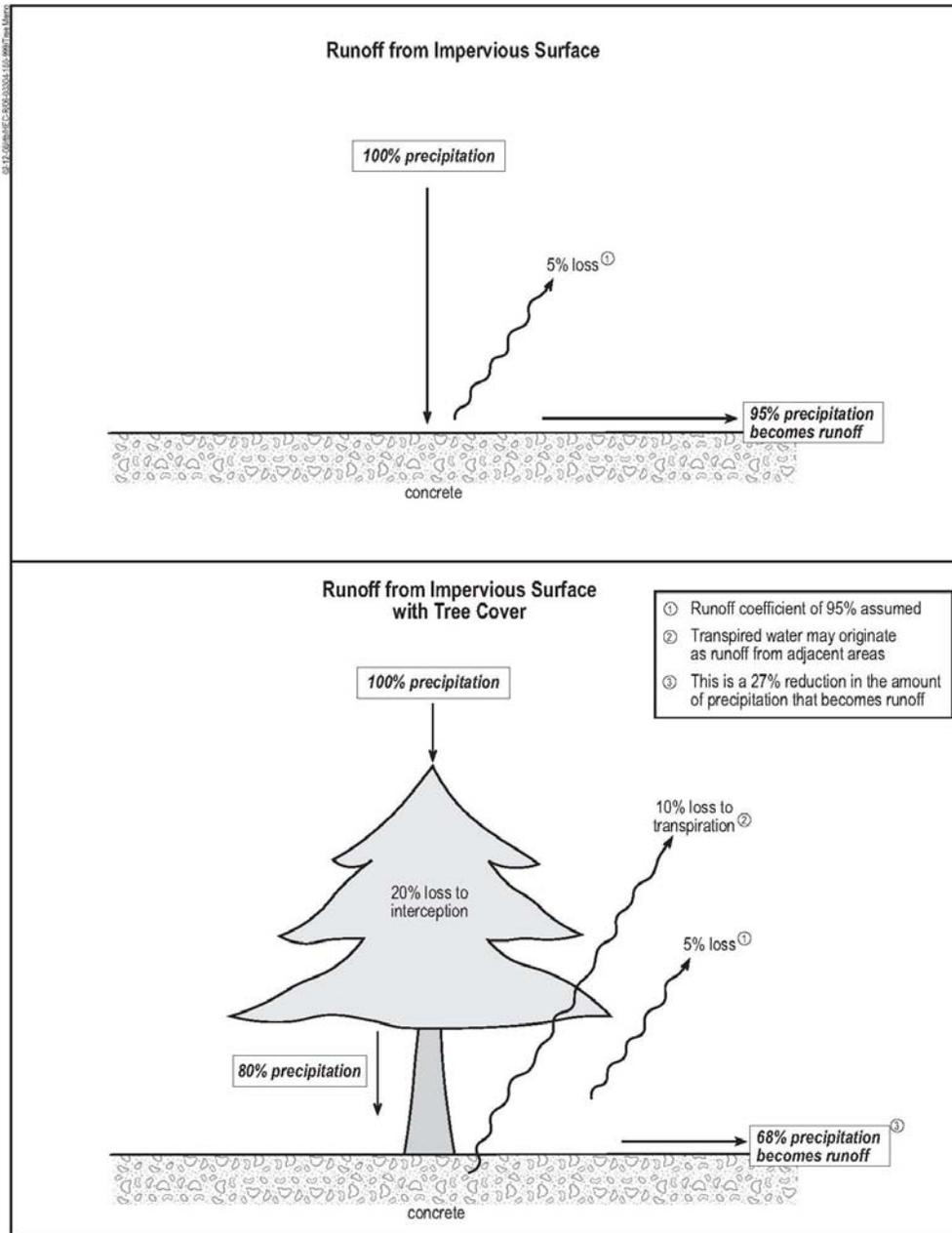
Figure 10.1: Conifer with underlying impervious surface versus impervious surface with no conifer.
