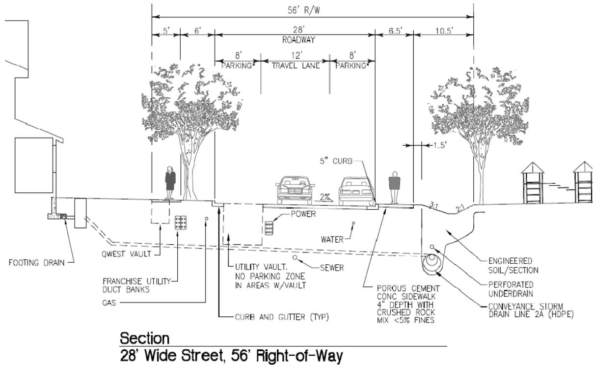
Figure 15.3: Section from High Point, West Seattle, showing electric utility vault location
