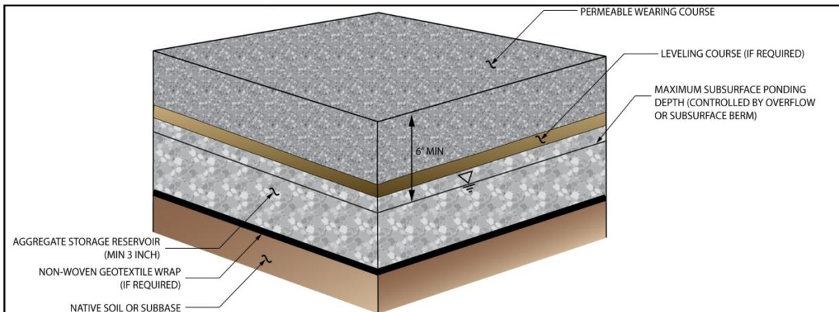
*Figure 1.3: Typical Permeable Pavement Facility Section - (Maximum ponding depth kept to a minimum of 6" below the surface of the wearing course to prevent saturation of wearing course and possible freeze/thaw damage)*
