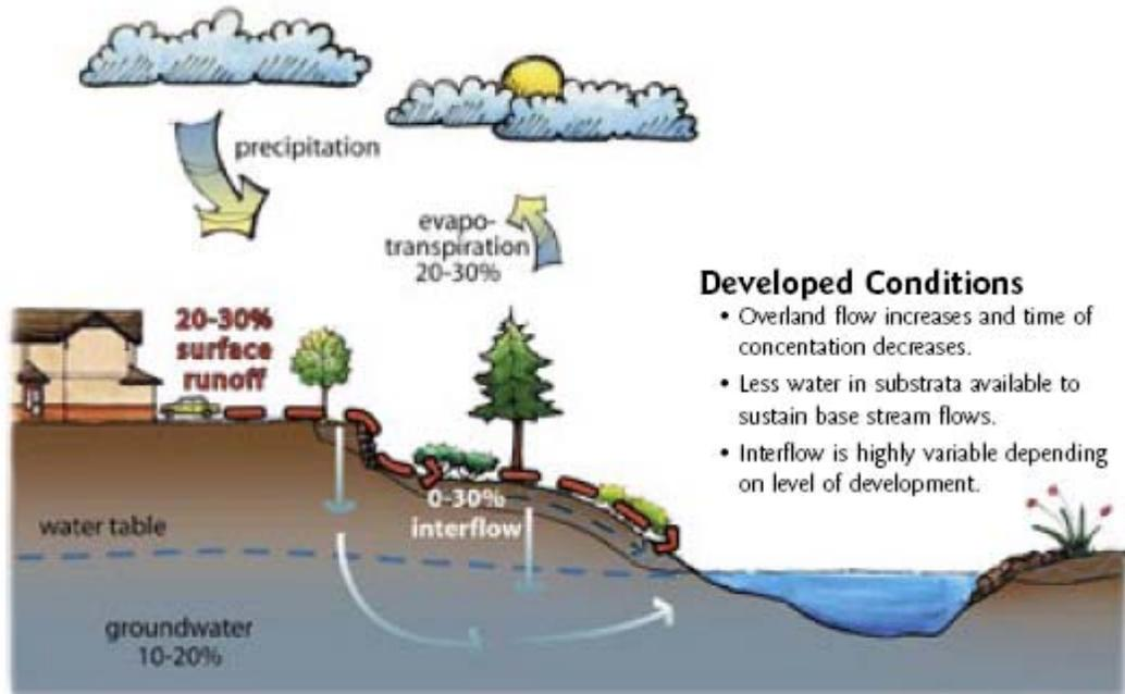
Fig 3 – Hydrological cycle for conventionally developed conditions in Puget Sound. Source: LID Technical Guidance Manual 2005
