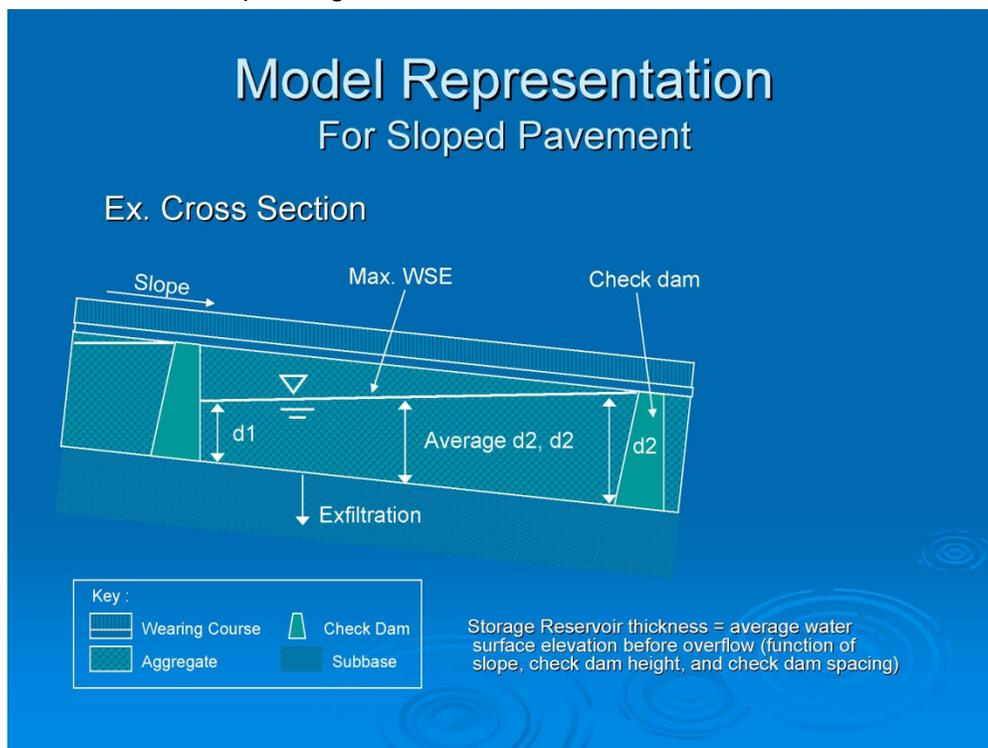
Figure 1.4: Modeling representation of sloped base storage with check dams
