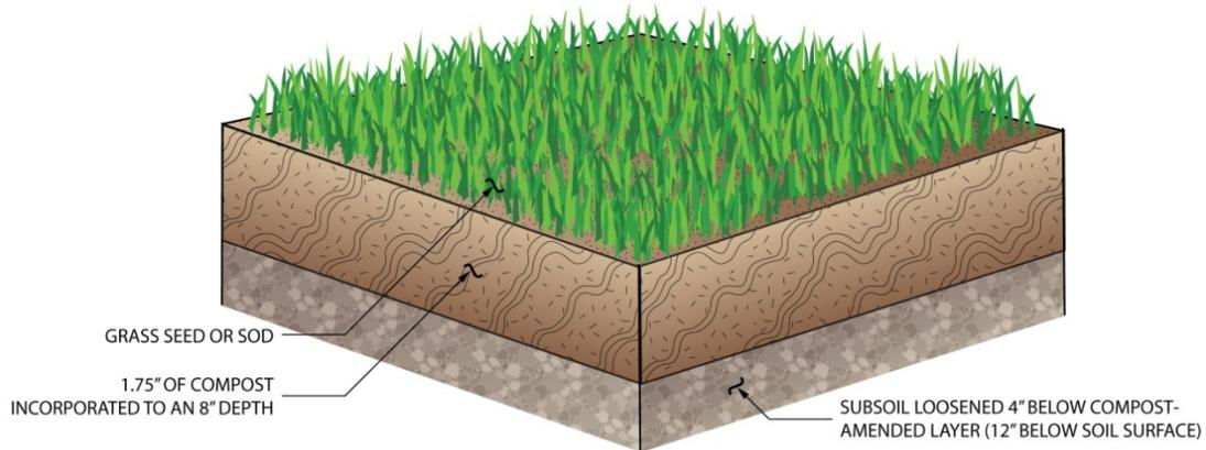
Figure 6.2: Cross Section of Turf Soil Amendment. (Source: Seattle Public Utilities/Seattle Department of Planning and Development)
