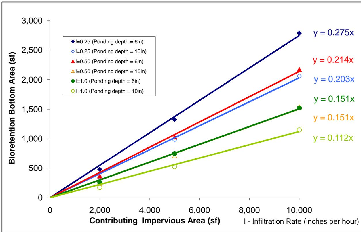
Figure C2. Bioretention facility (bottom area) sized for flow control as a function of contributing impervious area (annual precipitation of 36 inches).
