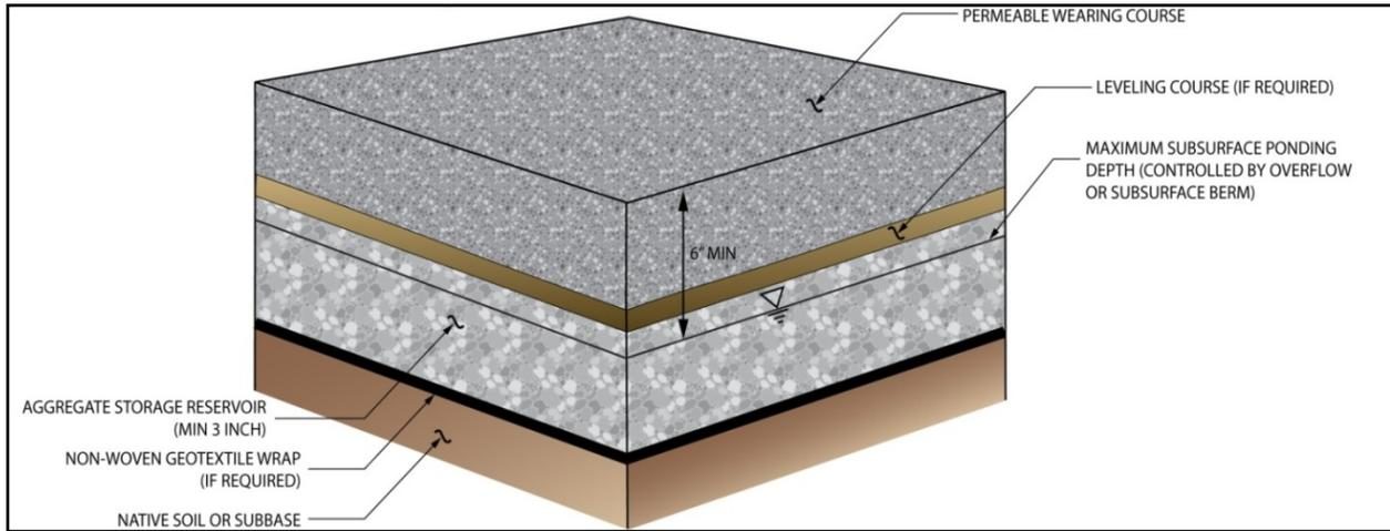
*Figure 2.2: Typical Permeable Pavement Facility Section – (Maximum ponding depth kept to a minimum of 6” below the surface of the wearing course to prevent saturation of wearing course and possible freeze/thaw damage)
