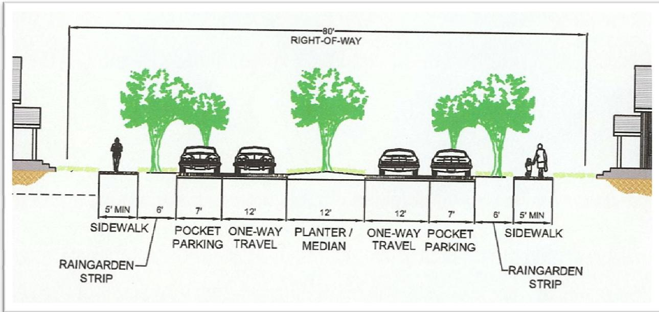
Figure 15.4: Example of “parkway” with narrow travel lanes and pocket parking with sidewalk separated by raingarden/bioretention strip for appeal, safety and stormwater sheet flow to facility.
