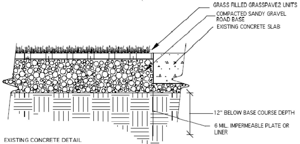
Figure 3.3: Typical section for cellular reinforced grass pavement adjacent to conventional impervious pavement. Source: NA
