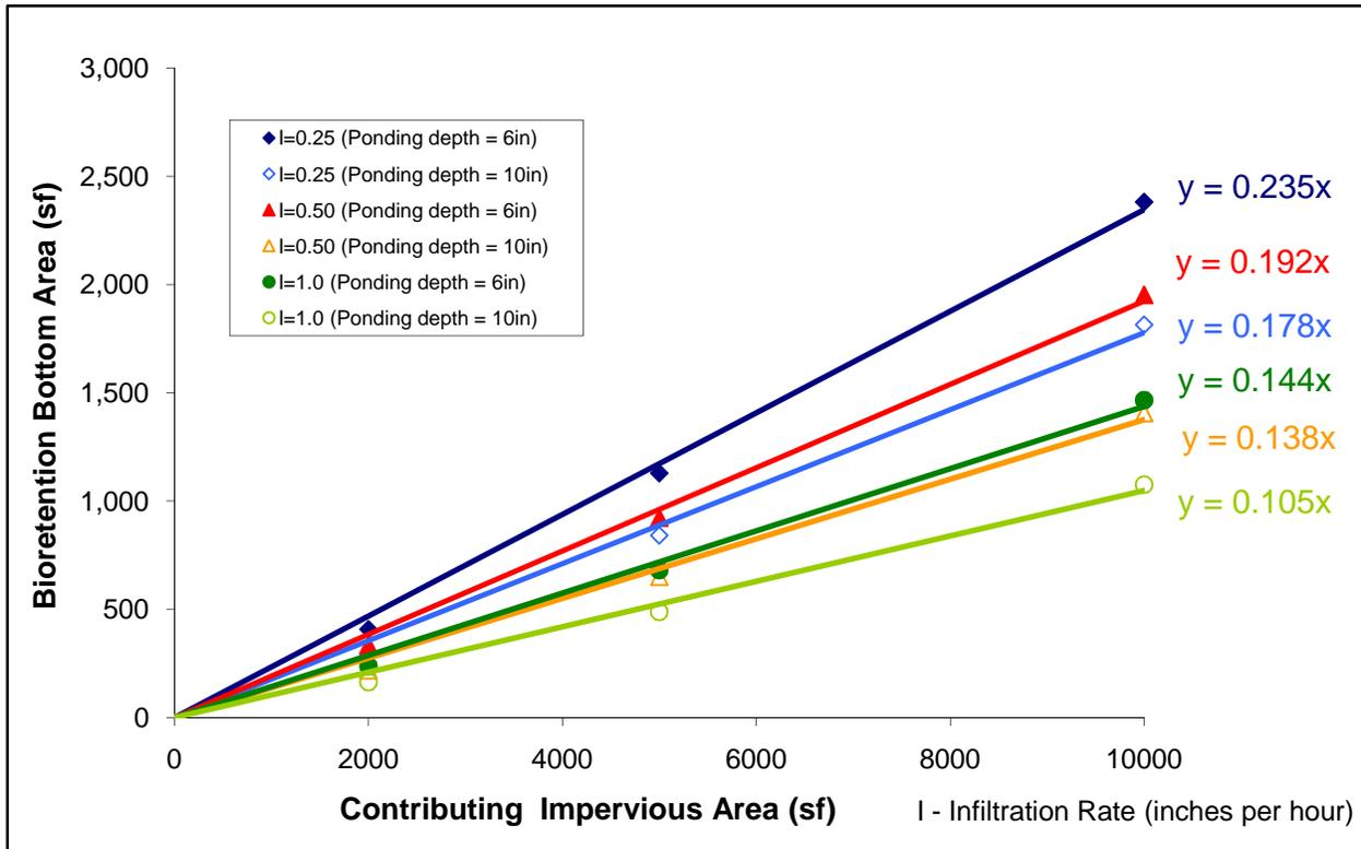
Figure C1. Bioretention facility (bottom area) sized for flow control as a function of contributing impervious area (annual precipitation of 32 inches).
