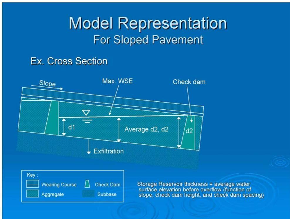
Figure 2.3: Modeling representation of sloped base storage with check dams
