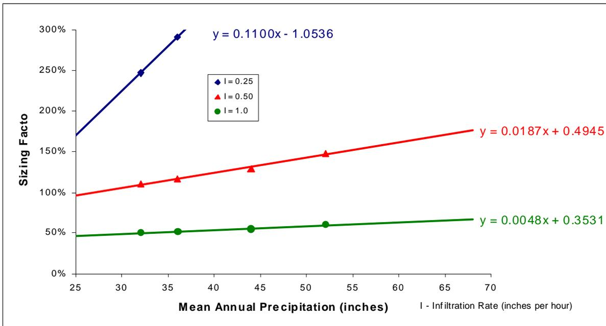
**Figure 6. Permeable pavement facility flow control sizing factors for Kitsap County as a function of mean annual precipitation.**
