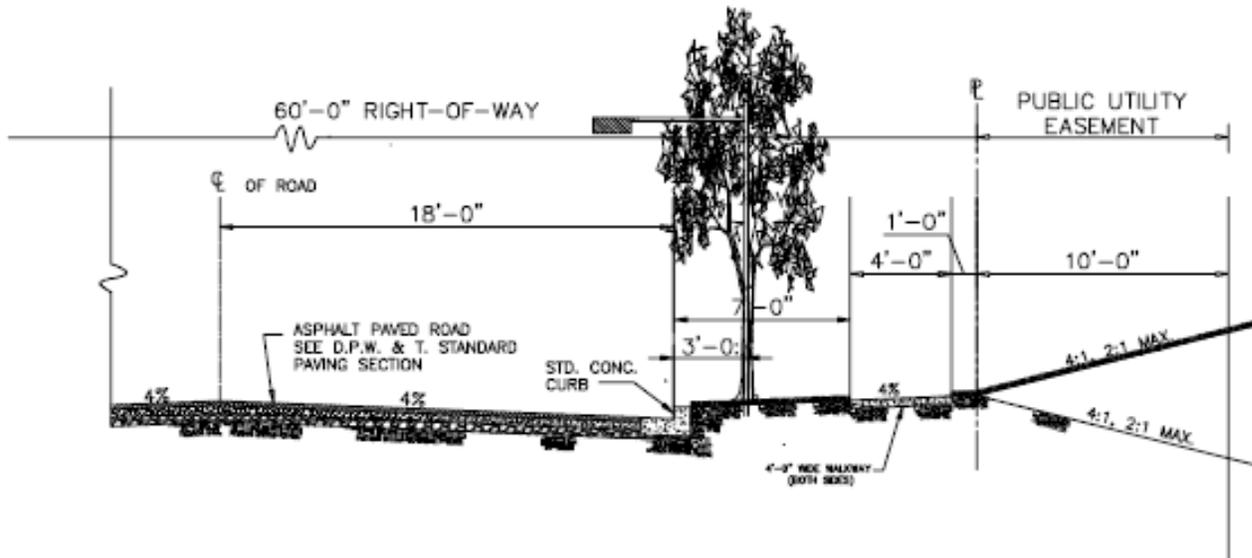
Figure 15.2: Example of a conventional right-of-way section with pavement width of 36 feet and use of concrete curb and gutter
