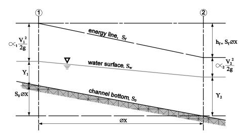
Use Equation F-9 to calculate the total head at cross-sections 1 and 2.
