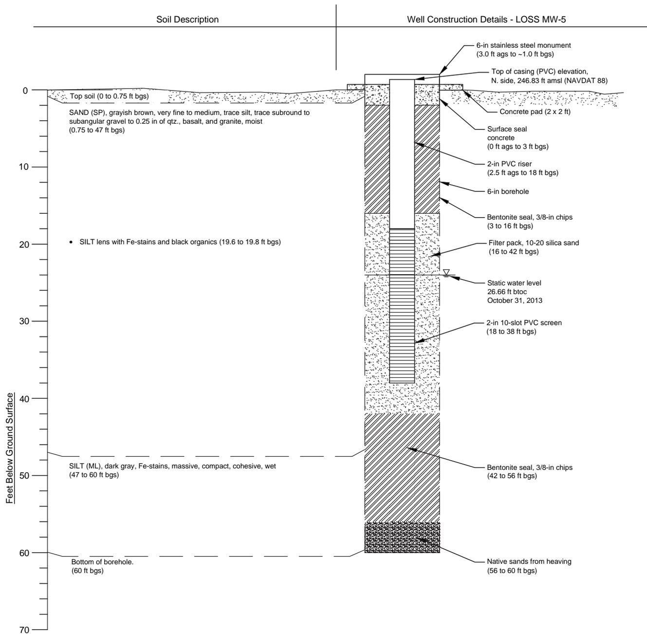
C:\Users\Craeburn\Desktop\CAD - working folder\Port Gamble Loss MWells\_v0.3.dwg | FIGURE 5 - LOSS MW-5 | Mod: 11/11/2013, 15:51 | Plotted: 11/11/2013, 15:52 | Craeburn
