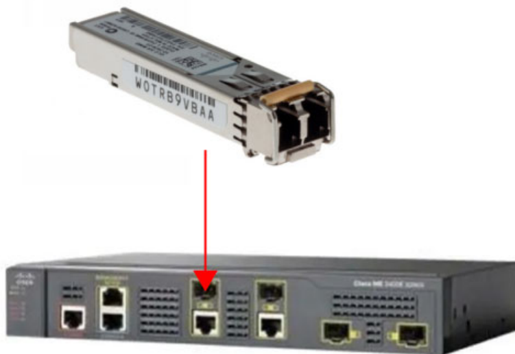
Figure 5-7. Proposed SFP module installation in KPUD Carrier Ethernet combination port
